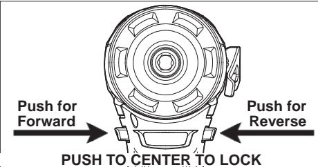
For **forward** (clockwise) rotation, push the control switch in the direction shown. Check the direction of rotation before use.
